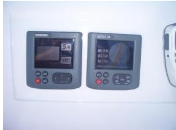
Log 5,4kn SOG 8,8kn = 3,4kn current
